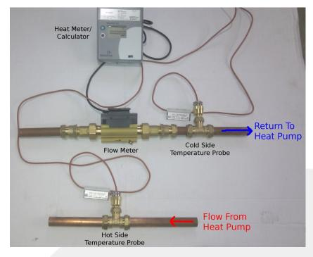
The probes should be positioned as close to the heat pump as possible. The pipe between probes and the heat meter should be well insulated. Do **not** reduce the length of the probe cables.
