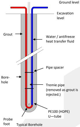
Along with the borehole pipe a small tremie pipe (25– 40mm) is also inserted attached to the borehole pipe. The tremie pipe is used to fill the borehole completely with thermal grout and is withdrawn as the grout is injected. The thermal grout provides an enhanced thermal path to allow the energy within the ground to be absorbed by the fluid circulating around the borehole pipe. The driller will take responsibility for grouting the hole using specialist pumping equipment.
