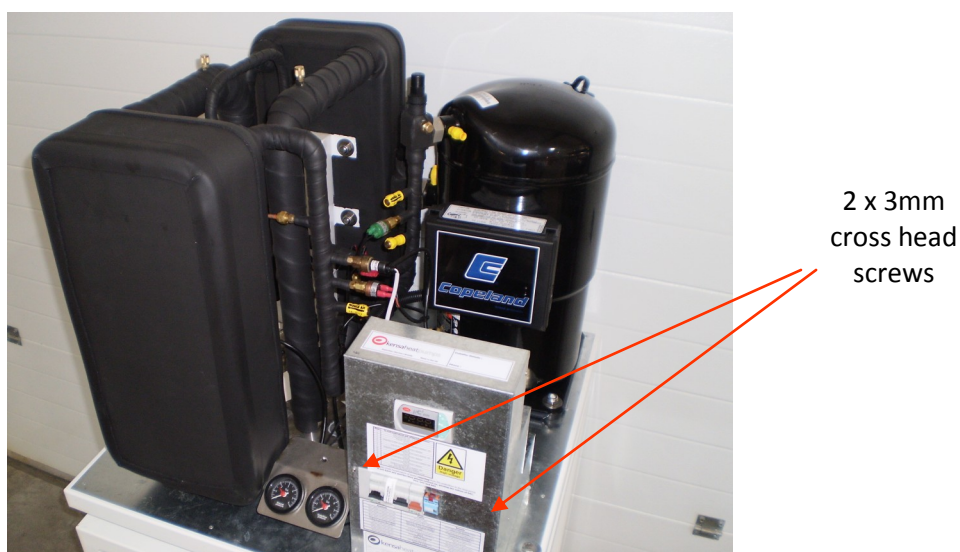
Fig 9 Position of hex screws on the electronics cover plate
