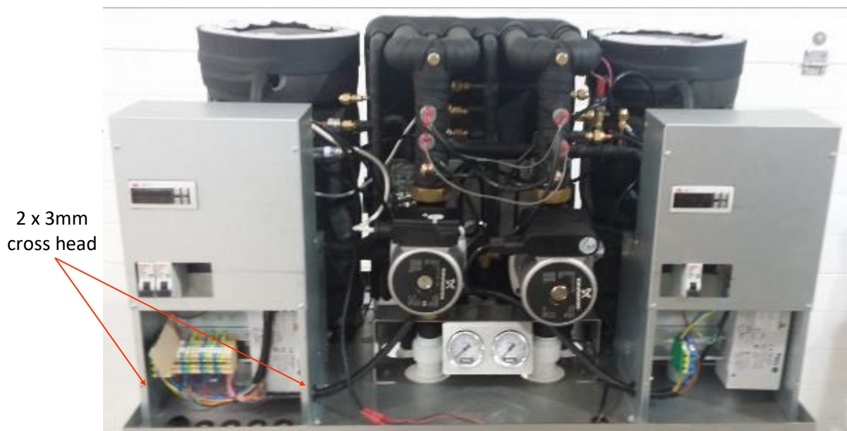
Fig 16 Position of Hex screws on the Electronics cover Plate
