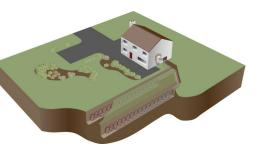
Straight pipe can also be used, however this can increase the amount of digging required by up to 5 times and hence the cost of installation. There is no difference in the amount of ground required as the energy source for slinkies or straight pipe and both have the same performance. Kensa heat pumps can work with both types of ground array and we can supply both. However due to the advantages of slinkies we would always recommend these.
