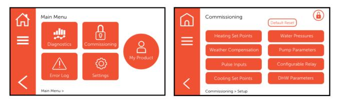
In commissioning mode the Pulse Input screen can be used to enter the 'name, pulse reading and unit.' (padlock in top right corner) For the Lovato you would enter 'Lovato, 10 and kWh' whereas the Finder you would enter 'Finder, 1000, kWh'.
