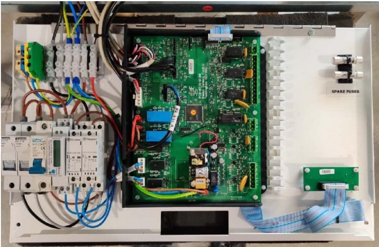
Fig 18 6kW Electrics panel folded down (lid removed from PCB box)
